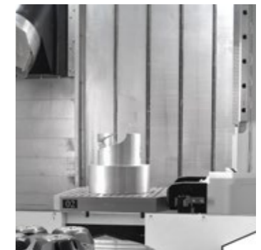
Pallet gripper: Positive locking system with pneumatic cleaning of the contact surfaces
